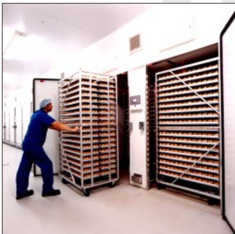
Loading a Chick Master Avida 12 single stage setter
